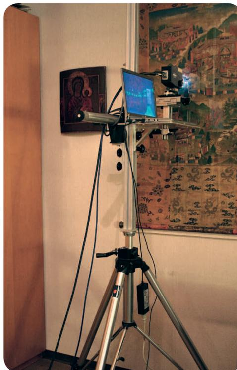
Figure 3: Raman Video Probe mounted on a tripod.
