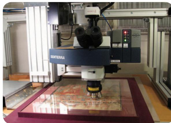
Figure 1: Raman microscope SENTERRA mounted on a gantry.
