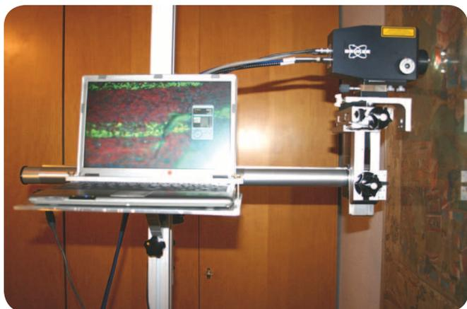
Figure 2: Raman Video Probe with laptop PC.
