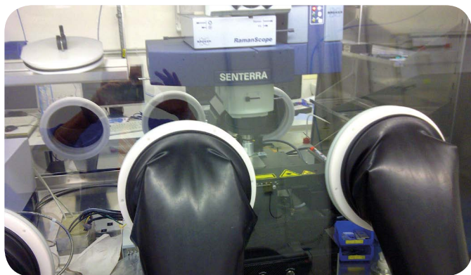
Figure 1: Raman microscope SENTERRA was installed into glove box, to analyze sensitive materials in an inert atmosphere. [2]
