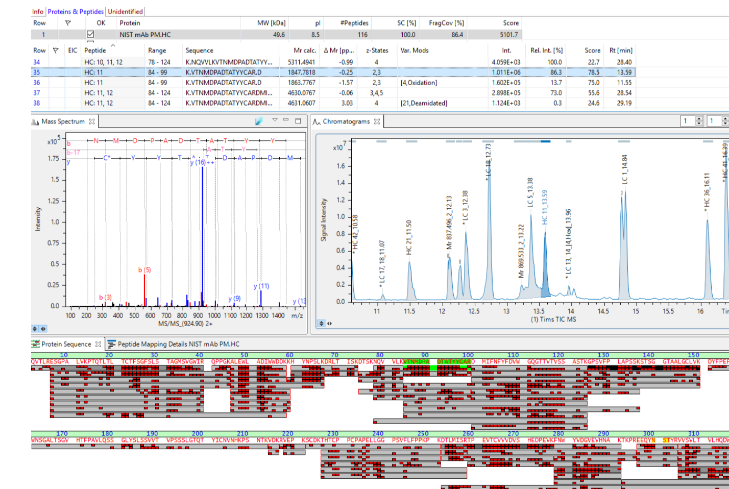
Figure 2. Peptide mapping search result. Top shows the identified proteins with corresponding peptide details. Modifications and relative modification ratios can be obtained; Middle is the MS/MS spectrum and the corresponding chromatogram; Bottom show the protein sequence coverage.
