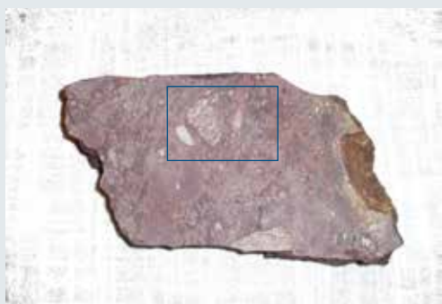
Fig. 1 The highlighted sample area was analyzed with Micro-XRF.
