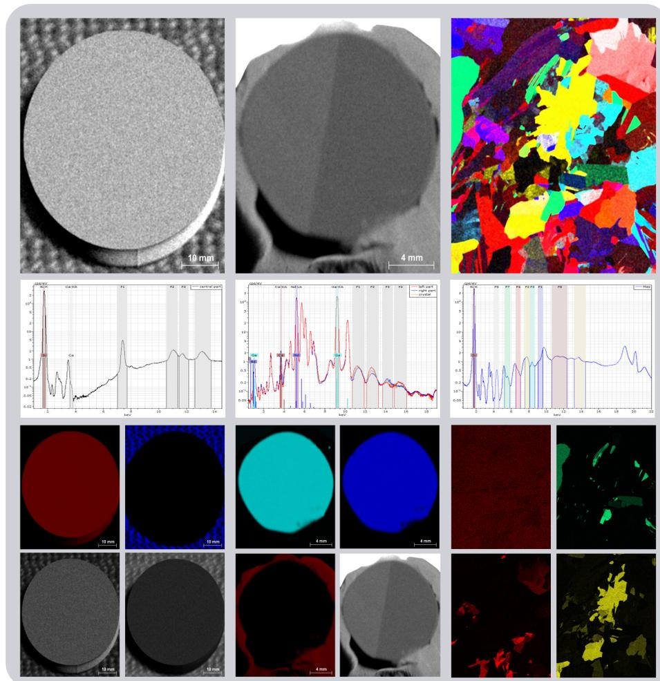
Fig. 3 Top row: Bragg diffraction peak distribution along the scanned sample surface. Middle row, sum spectra and selected energy regions (ROIs). Bottom part: element and Bragg peak intensity distributions.
