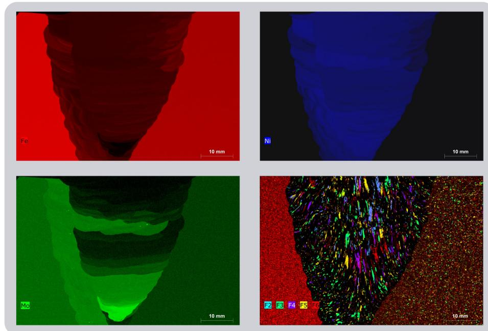
Fig. 4 Element map and diffraction pattern distribution of a large welding joint (70 mm x 50 mm). Two different steels were welded using a Ni rich welding consumable. The crystallization hints to the temperature gradient during and after the processing.
