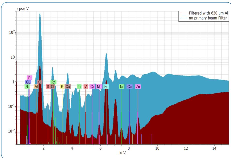
Fig. 2 Sum spectrum of a multi crystalline Si with impurities measured with (red) and without (cyan) primary beam filter. Trace and minor elements can only be quantified when diffraction is suppressed. The detected intensity is dramatically reduced.
