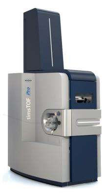
The timsTOF Pro uses trapped ion mobility spectrometry (TIMS), where ions are propelled through the TIMS tunnel by a gas flow. An electrical field controls each ion from moving beyond a position defined by the ion's mobility, where the push it experiences from the gas flow matches the force of the electrical field. Ramping down the electrical field allows selectively releasing ions from the TIMS tunnel according to their mobility.
