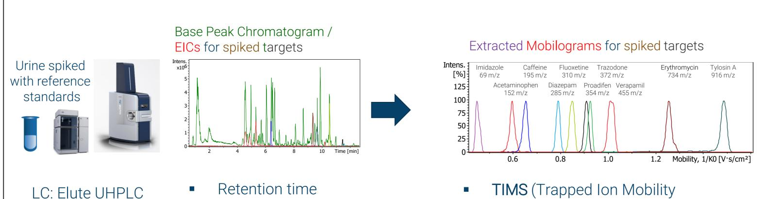
TIMS (Trapped Ion Mobility Separation)= reproducible CCS values The novel data acquisition utilizes TIMS stepping and provides broad profiling and screening/quantitation in a single acquisitions for target samples.
