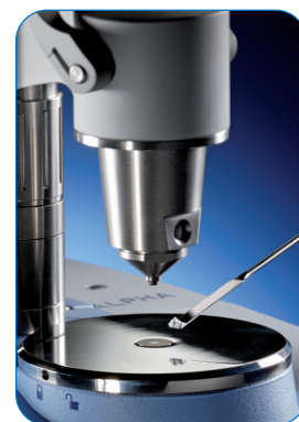
Figure 1: ALPHA II FTIR spectrometer with optional touch-PC (left) and powdered sample being placed on the Platinum ATR accessory (right).
