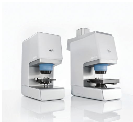
Fig. 3 LUMOS II stand-alone FT-IR imaging microscope
