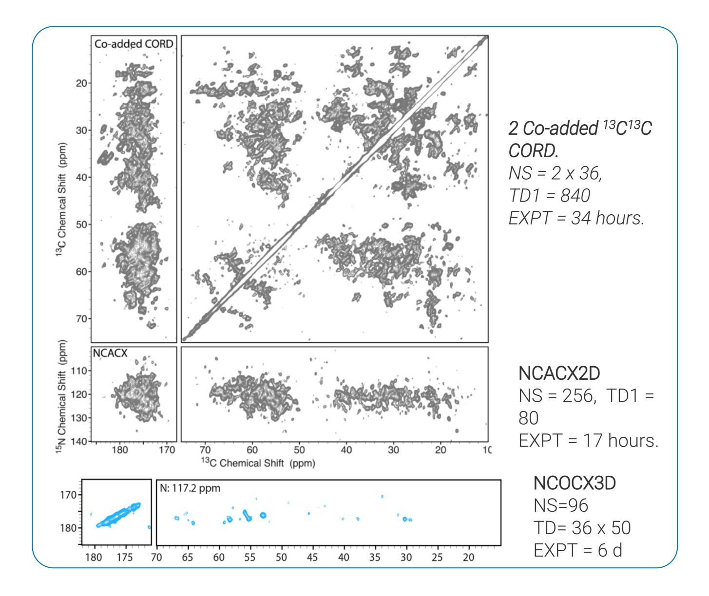
The new CP-MAS CryoProbe proved essential for the analysis of drug binding in the sponge like structure of a cyclodextrin-based metal-organic framework, loaded with a small amount of drug (Lansoprazole). The natural abundance <sup>15</sup>N CPMAS NMR spectra of this extremely dilute sample, showed clearly that the LZP is deprotonated upon loading into the CD-MOF (C. Martineau, (Int. J. Pharm. 585) (2020) 119442)).
