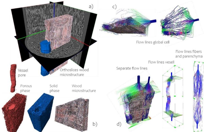
Figure 1: a) 2D multi ortho slices and 3D rendering of the vessels and wood's microstructure. b) 3D rendering of the different elements that compose the wood's microstructure. c) and d) Simulated flow lines throughout the porosity of the *Dalbergia ruddae* wood.
