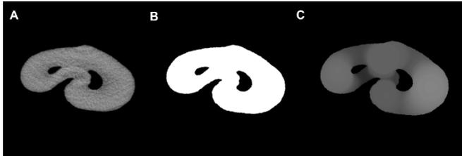
**Figure 1.** Processing and analysis of reconstructed images in CTAn software. (A) Original reconstructed image. (B) Binarized image. (C) Binarized image based on 3D mapping of the dentin thickness.
