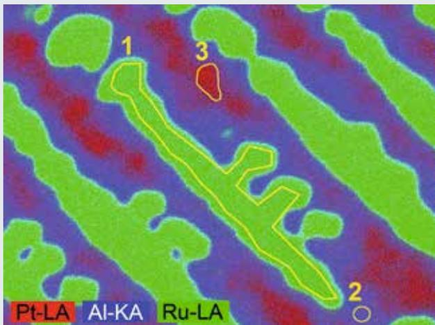
Fig. 2 Composite element map of Al-K $\alpha$  (blue), Ru-L $\alpha$  (green) and Pt-L $\alpha$  (red). Numbers correspond to three differently composed areas (1: ruthenium-enriched crystals, 2: matrix with less platinum, 3: platinum-enriched matrix).
