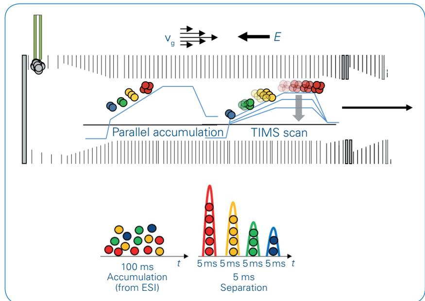
Figure 2: Confinement and release of the ions within the tims cell. All ions accumulated for 100 ms are concentrated in 5 ms width Ion Mobility Separated peaks, ensuring a dramatic increase in both acquisition speed and sensitivity. The dual tims cell architecture allows for parallel accumulation with close to 100% duty cycle: ions are still accumulated in the first cell as they are released from the second cell.
