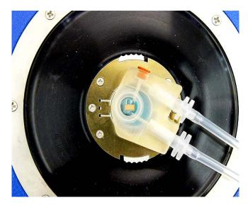
Fig. 2 The small volume SmallCell<sup>™</sup> takes the place of the standard tip holder
