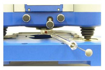
Fig. 3 Valuable solutions can be injected directly into the cell through the septum in the third port.
