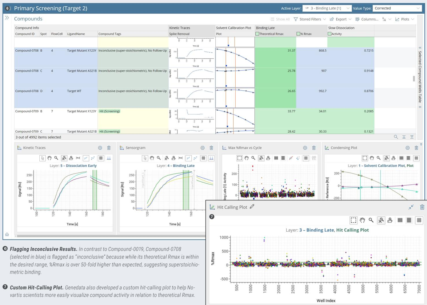
**6 Flagging Inconclusive Results.** In contrast to Compound-0019, Compound-0708 (selected in blue) is flagged as "inconclusive" because while its theoretical Rmax is within the desired range, %Rmax is over 50-fold higher than expected, suggesting superstoichiometric binding.
