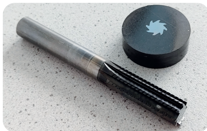
Figure 1: The carbide cutter (bottom left) with a cross section embedded in resin (top right).
