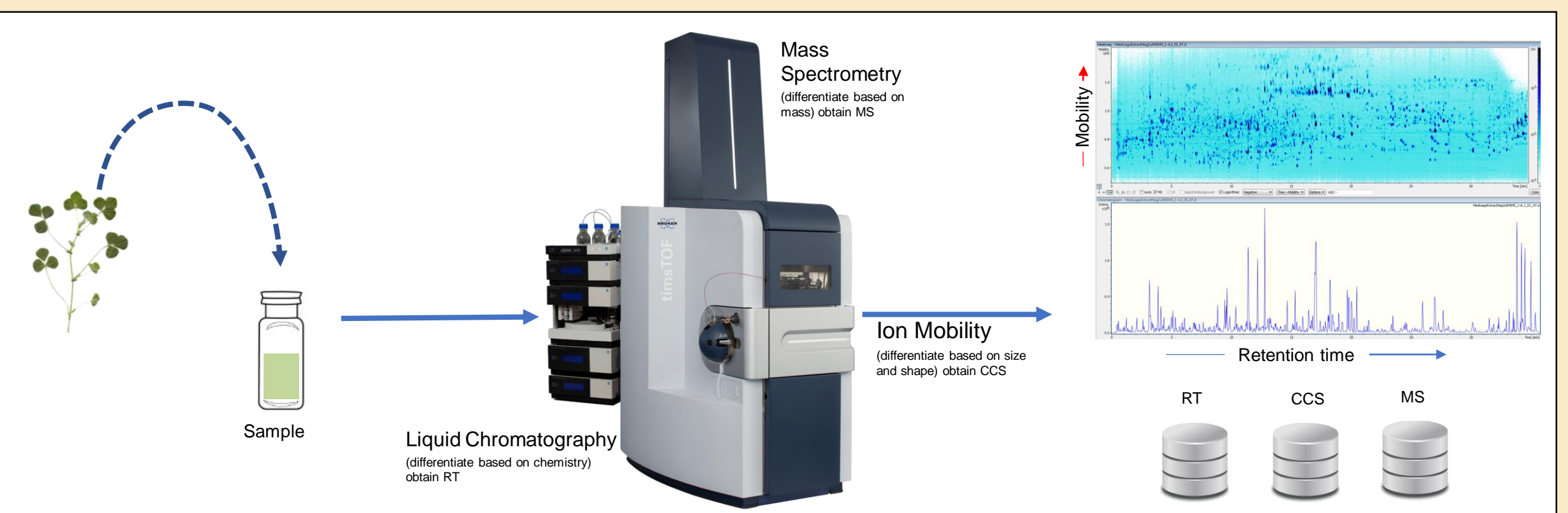
Fig. 1. General LC-TIMS-MS metabolomics workflow. Sample is prepared, LC, TIMS, and MS data are acquired. Data is then compared with reference databases.
