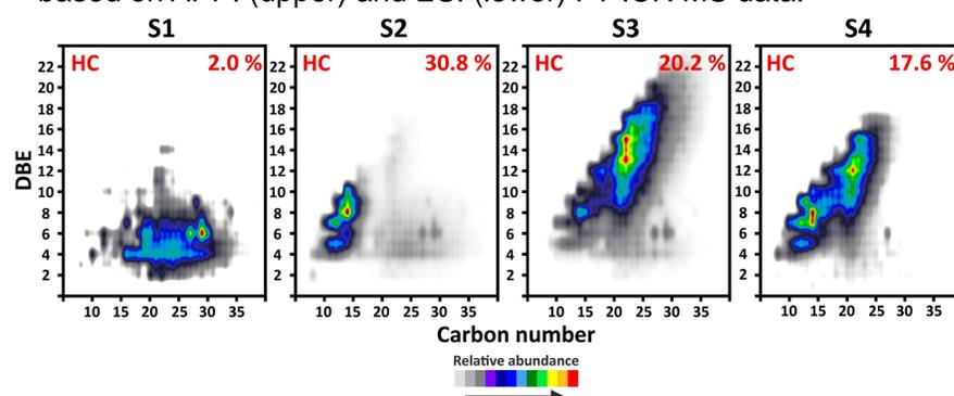
**Figure 3.** Isoabundance contour plots of double bond equivalent (DBE) versus carbon number for the HC class compounds (only radical cations) by APPI FT-ICR MS.
