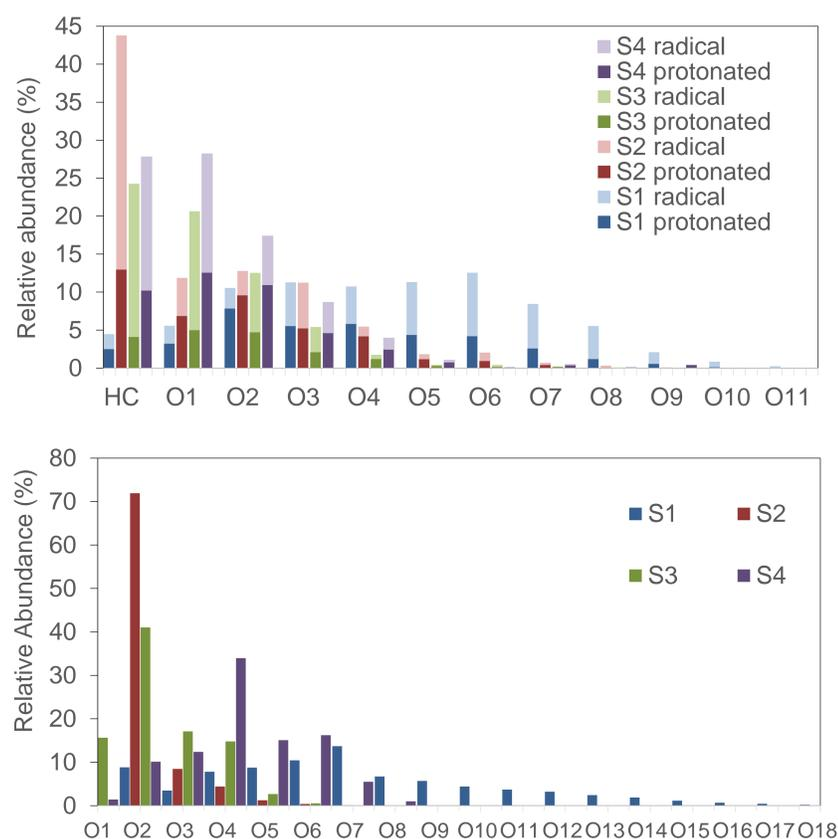
**Figure 1.** Heteroatom class (HC and O<sub>y</sub>) distributions by APPI (upper) and ESI (lower) FT-ICR MS. Minor N<sub>x</sub>O<sub>y</sub> and S<sub>z</sub>O<sub>y</sub> classes are omitted.
