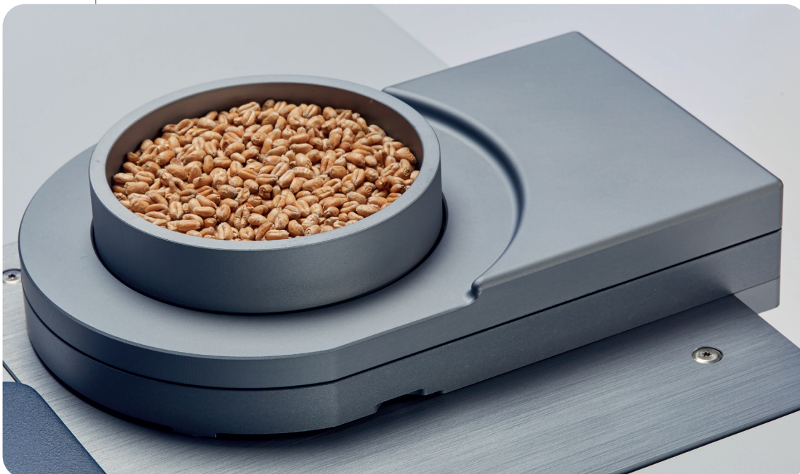
Analyzing feed ingredients (here: wheat) with in an aluminium cup with quartz glass bottom using the MPA II FT-NIR spectrometer
