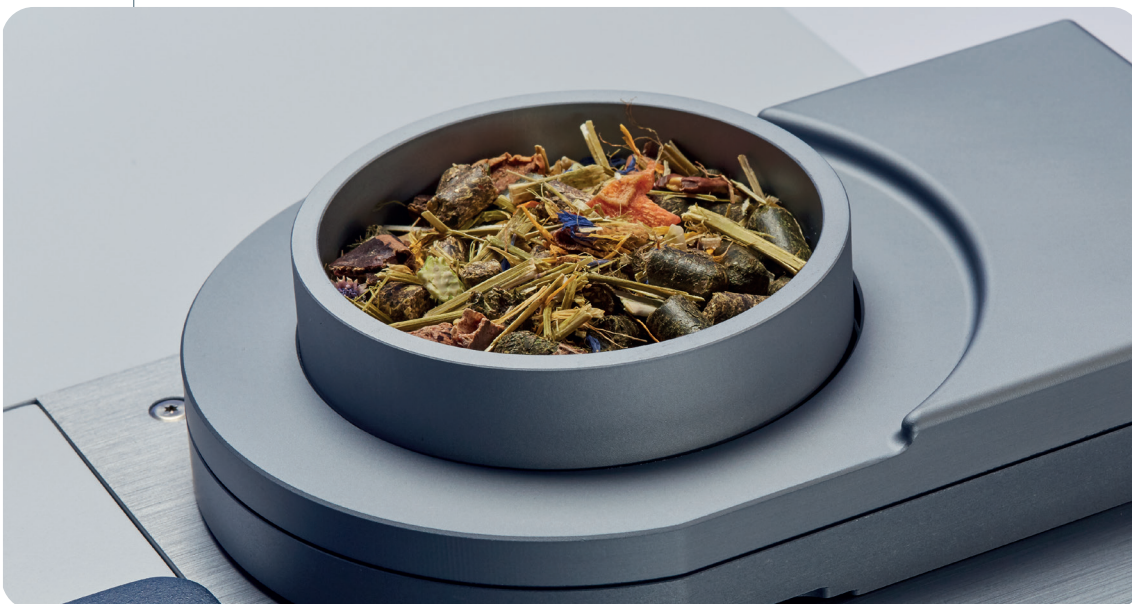
Analyzing rabbit food in an aluminium cup with quartz glass bottom on the MPA II FT-NIR spectrometer
