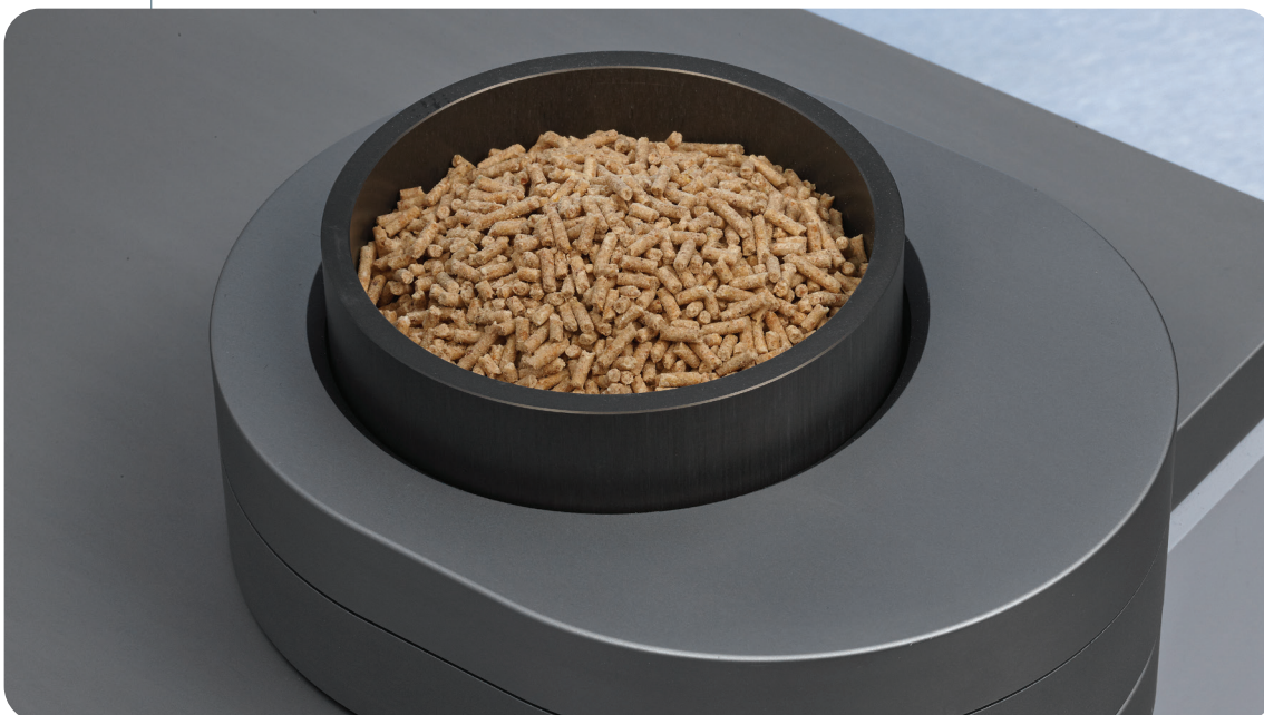
Analyzing feed pellets in an aluminium cup with quartz glass bottom on the TANGO FT-NIR spectrometer
