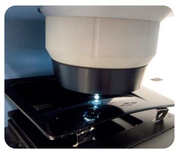
Figure 5: Louver on the sample stage.
