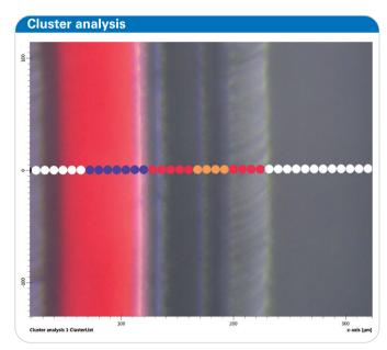
Figure 2: Cluster analysis of the composite film. Example spectra are shown in figure 4.
