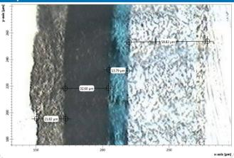
Figure 5: Layer thickness determination in transmission.
