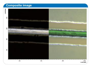
Figure 9: Visual composite image. Left without and right with polarizers.
