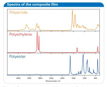
Figure 4: Representative spectra of the composite film in the respective colors of figure 2.
