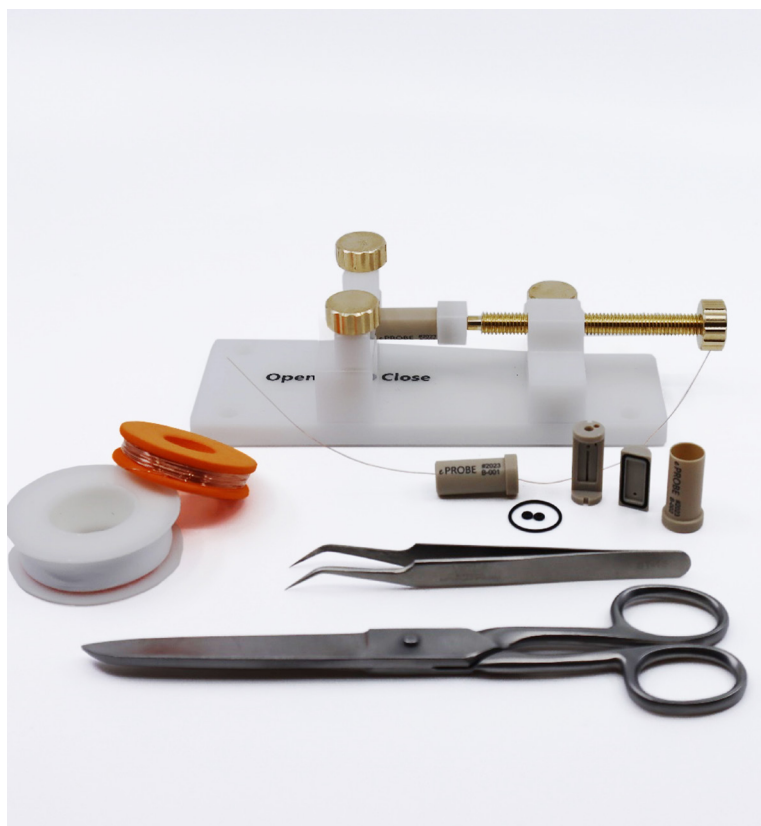
In-situ battery cell set, consisting of plastic cell capsules, an assembly and disassembly tool and various accessories
