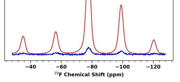
**Fig.1** <sup>1</sup>H/<sup>19</sup>F CP-MAS spectra, with & without DNP, of NH<sub>4</sub><sup>+</sup> trifluoro acetate. <sup>1</sup>H DNP gain (on/off): 250x. Sample plus 12 mM AMUPol radical in (60/30/10) glycerol-d<sub>8</sub>/D<sub>2</sub>O/H<sub>2</sub>O, 3.2 mm rotor, 8 kHz MAS, 9.4 T  $(400 \text{ MHz} {}^{1}\text{H}), T = 106 \text{ K}.$
