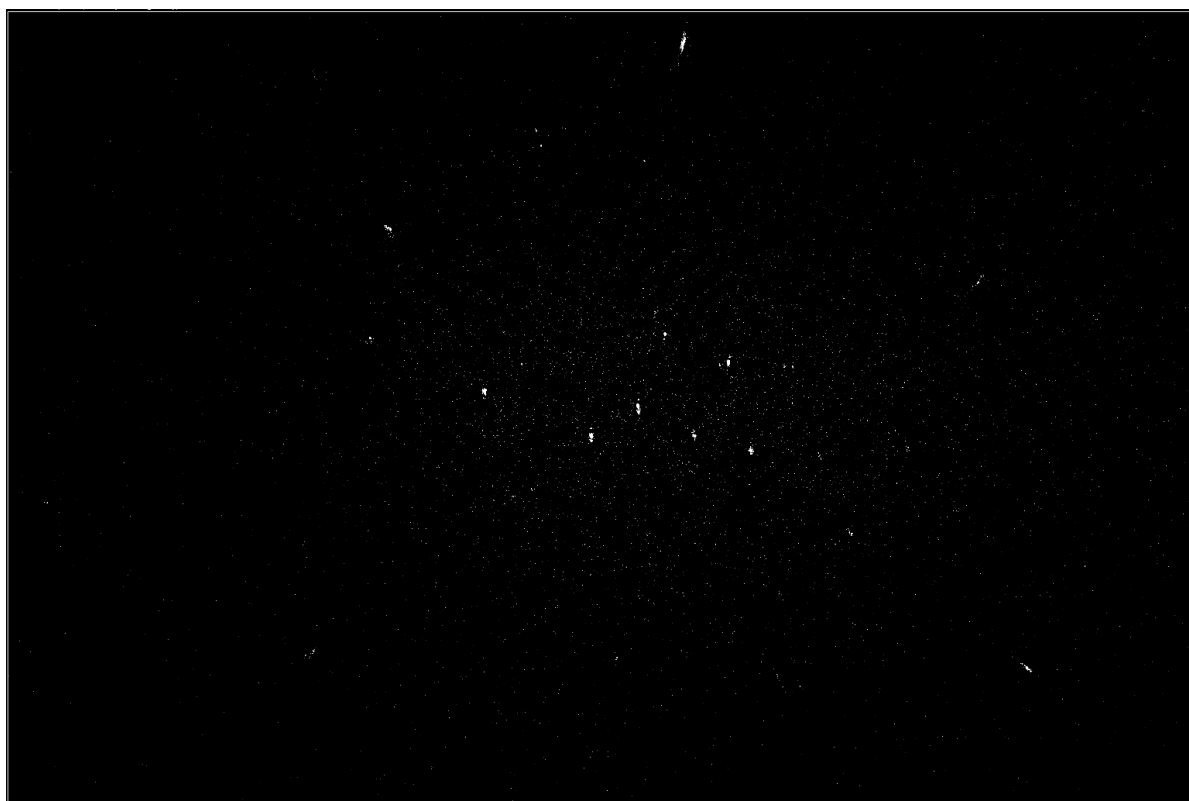
Figure 3. A 1 second composite exposure obtained by summing 70 individual exposures (diffraction from the same sample as in Figure 2). Individual Bragg reflections can be seen in the composite image. Note that at high resolution, where there are few scattered X-rays there is essentially no background noise in the composite image.
