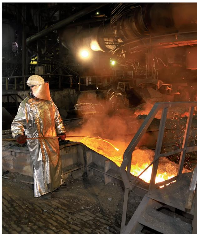
Figure 1: Sampling of slag in a steel production plant .
