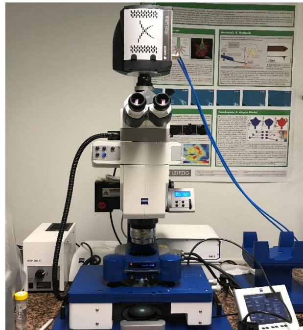
Fig. 2: JPK HybridStage on a Zeiss upright AxioZoom V.16 fluorescence microscope with an Andor EMCCD camera for force mapping experiments on non-transparent tissue samples.
