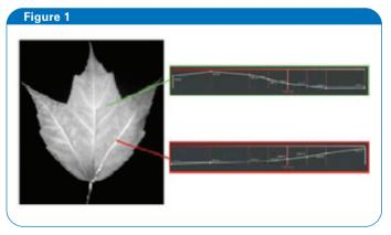
Spectral unmixing of indocyanine green and autofluorescence emission signals from a sycamore leaf. The spectra in the green box represent the emission spectra of the leaf autofluorescence, while the spectra in the red box is the fluorescence emission spectra from indocyanine green in the leaf vasculature.
