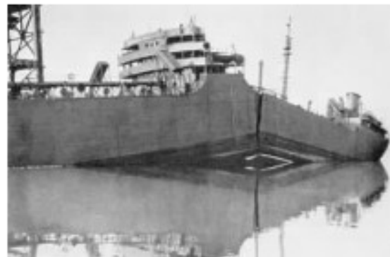
Figure 13: Liberty ship with brittle fracture
