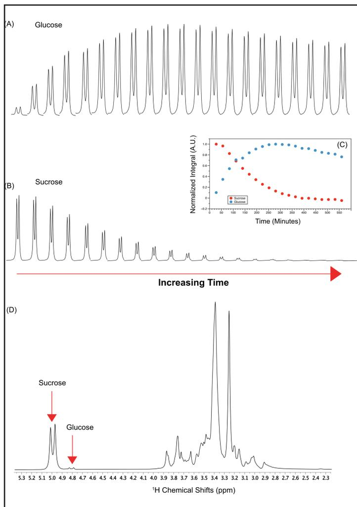
**Figure 2.** (A-B) A series of NMR spectra as a function of time showing only the anomeric doublet of the (A) glucose and (B) sucrose. (C) A graph of normalized integrals of sucrose and glucose as a function of time. (D) A spectrum showing a mixture of glucose and sucrose during enzymatic hydrolysis reaction.
