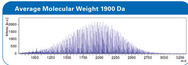
**QC analysis of co-polymers using MALDI-TOF MS system.** Co-polymer consisting of PEG and PPG: PEG-block-PPG-block-PEG.
