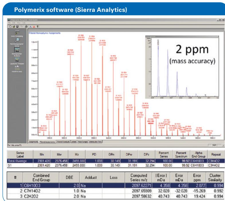
**QC analysis of poly(lactic acid) on an autoflex max MS system.** Monomer units are easily verified, and the overview spectrum (ext. calibration) indicates that polymerization occurred from both monomer and dimer species. The combined end group is identified as C<sub>6</sub>H<sub>10</sub>O<sub>3</sub>, with mass accuracy within 2 ppm.
