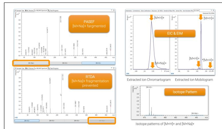
**Figure 2. Positive effect of the RTDA plugin for a feature detected across all replicate measurements.**
