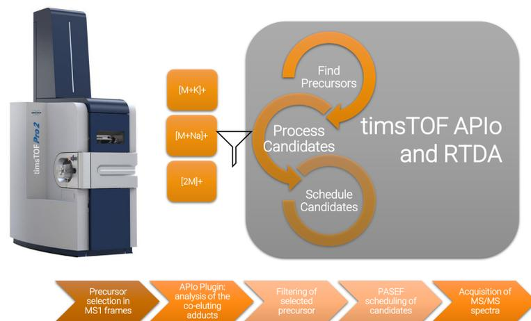
**Figure 1. Real time API prototype to control PASEF precursor selection**
