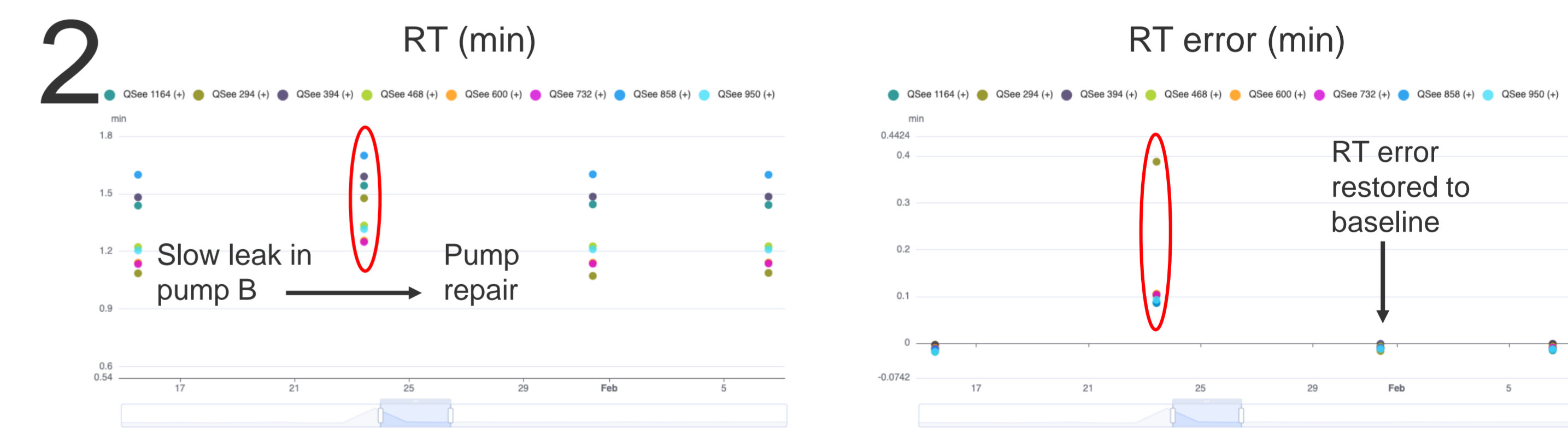
Figure 4: 1) Reduction in peak area due to Front-End contamination, areas restored after cleaning 2) Retention time deviation in a singular QSee run allowed for identification of a minor leak in pump B, RT is restored to baseline after cleaning of check valve
