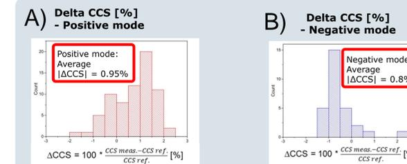
**Fig. 5** Deviation of CCS values measured on a timsTOF Pro versus CCS values from the public CCS Compendium repository [6].
