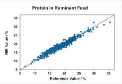
Calibration models: Models shown here display validation results for two example raw materials.
