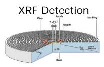
Silicon Drift Detector with XFlash® Technology
