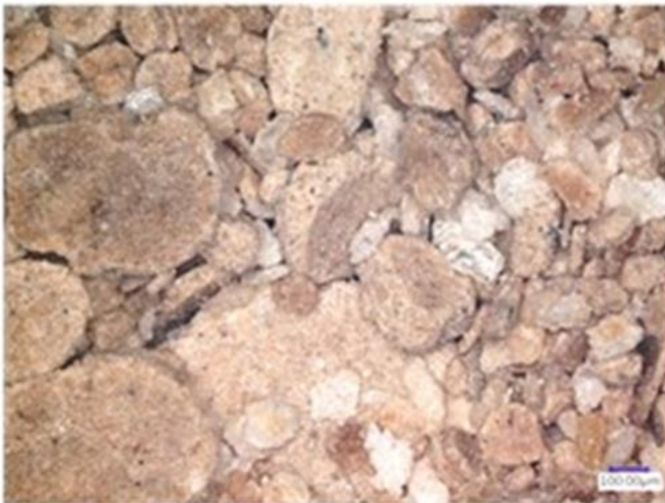
Speed: 1100 rpm Fraction X \geq 75 \mu m
