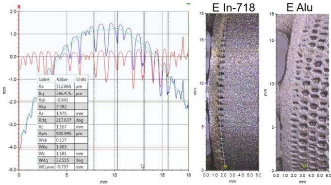
Figure 1: Extraction of shape, waviness and roughness on Inconel powder manufactured ring by LSM. Right hand image shows corresponding part made from aluminium
