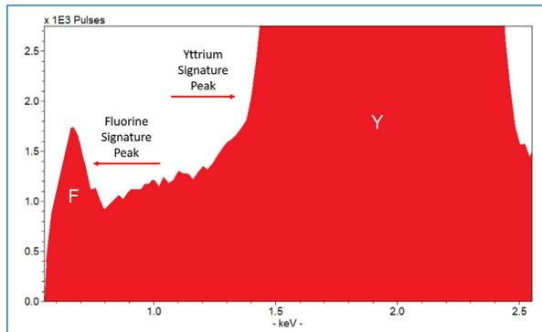
Yttrium fluoride (YF<sub>3</sub>) coating measurement with TRACER 5g
