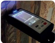
**Handheld Raman Compound Analyzer:** *BRAVO™ is the most nimble Raman spectroscopy analyzer from Bruker Optics. This handheld determines molecular content of inorganic and organic compounds with spectral databases identifying unknown materials including the most common pigments, fillers, binders and waxes available.*
