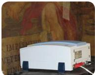
**Portable FT-IR Compound Analyzer:** *ALPHA II™ is an on-the-go FT-IR analyzer from Bruker Optics. It identifies molecular structures and components to help determine optimum cleaning methods and solvents with spectral databases of available varnishes, fibers and solvent which help guide restoration treatments without transporting valuable samples.*
