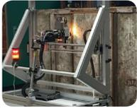
**Mobile 2D/3D Micro XRF Elemental Analyzer:** *M6 JETSTREAM™ μ-XRF and CRONO™ from Bruker Nano Analytics with motor-driven X-Y-Z positioning stage simultaneously measures elements from sodium (Na) to uranium (U) at concentrations as low as ppm to high percentage levels. Variable spot sizes from 100-500 μm with speeds up to 100 mm/s (M6) and from 500 μm - 2 mm with speeds up to 40 mm/s (CRONO) provide elemental distribution maps.*
