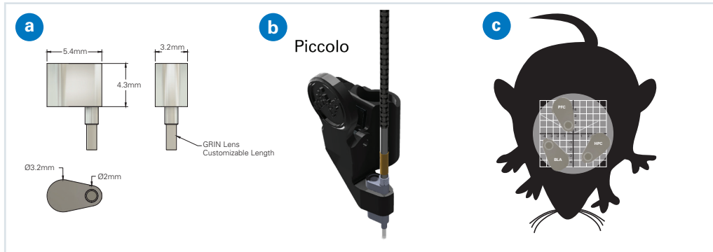
FIGURE 4. (a) Dimensions of a short and long GRIN lens with their protective caps on. (b) Piccolo® surgical accessory. (c) Diagram of the tear shape design enabling fitting multiple GRIN lenses on the head of a mouse.
