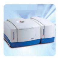
minispec mg20 polymer Analyzer for a wide range of polymer applications.
