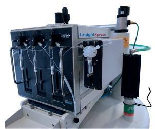
InsightXpress is a stopped–flow solution consisting of a pumping unit, a temperature controlled transfer line, a flow tube and software. The system is designed for seamless set-up in Bruker high-resolution NMR spectrometers with shielded magnets (300-700 MHz). Bruker's InsighMR<sup>TM</sup> software makes acquisition and analysis straightforward. It now has new functionality to enable the monitoring of very fast reactions.
