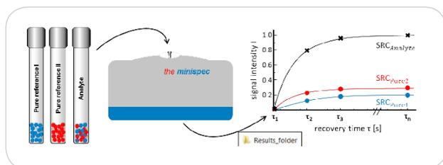
In the Dynamics Center, the SRCs are automatically fitted using the patent-pending linear-combination approach to reveal the relative mass percentages of the reference components in the analyte.
