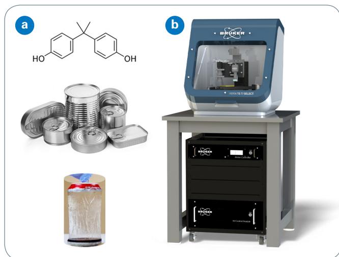
Figure 1. (a) Representative food and beverage can liner images; and (b) Bruker's Hysitron TS 77 Select benchtop indenter.
