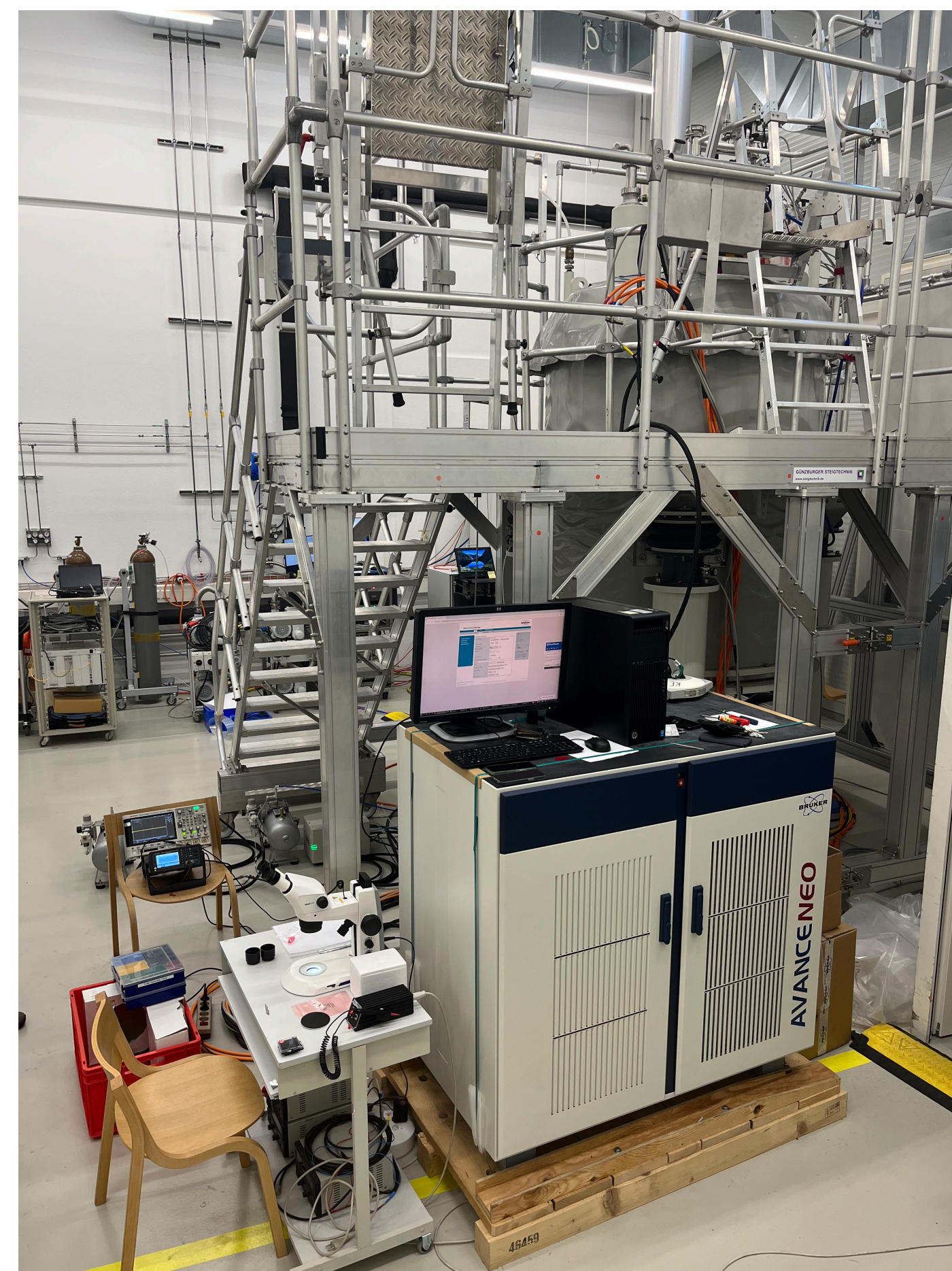
Fig. 1: The first-of-a-kind 1.3 GHz NMR magnet capitalizes on Bruker's well proven HTS/LTS hybrid technology.
