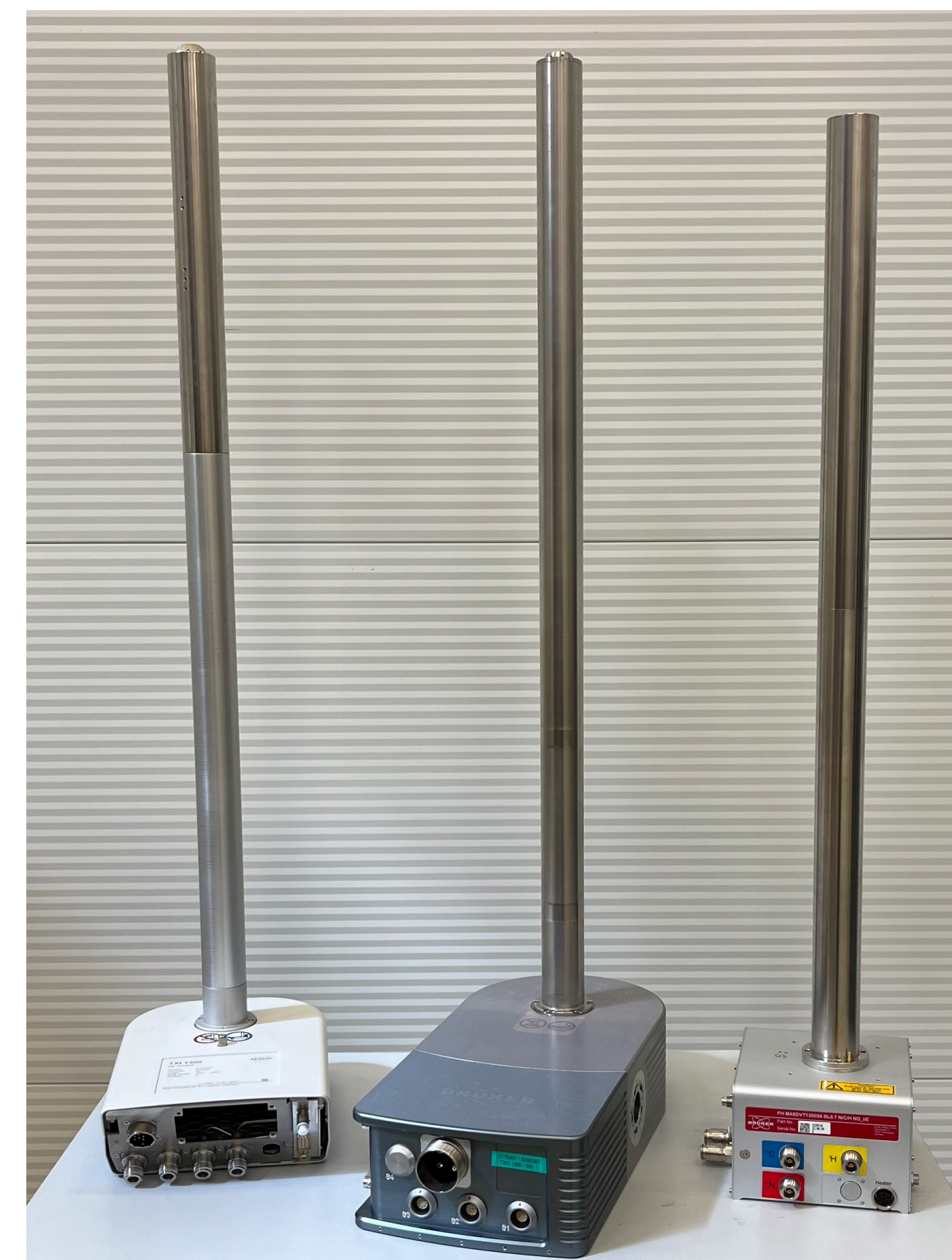
Fig. 2: Three of the NMR probes which were used for the first characterization of the 1.3 GHz spectrometer.
