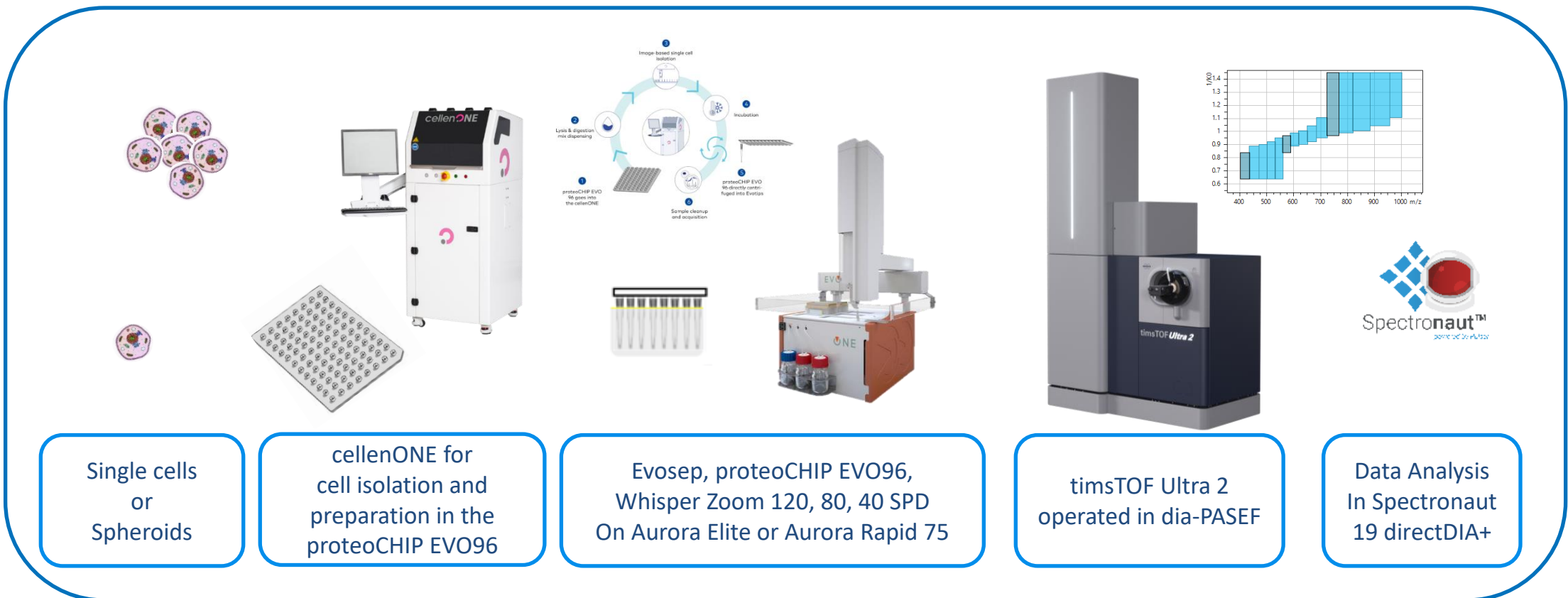
Figure 1: Single cell proteomics workflow with the Evosep One with Whisper Zoom 120, 80, and 40SPD using the proteoCHIP EVO96 for pipetting-free sample transfer onto Evotips Pure and pyDIAid [1] optimized dia-PASEF data acquisition on timsTOF Ultra 2 with data analysis in Spectronaut 19 .
