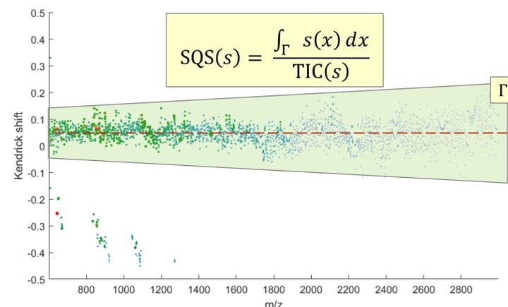
**Fig. 1** Kendrick plot of a peptide imaging spectrum using an appropriate Kendrick scale. Signal quality score (SQS) is computed as the relative total ion count (TIC) in the horizontal peptide corridor  $\Gamma$ . Location and shape of  $\Gamma$  is adapted to the data [1].
