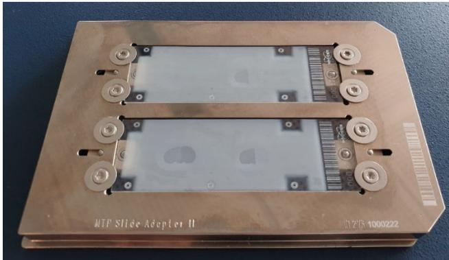
**Figure 3-3** Example of IntelliSlides™ coated with matrix using the modified mask, showing barcode and teachmarks free of matrix
