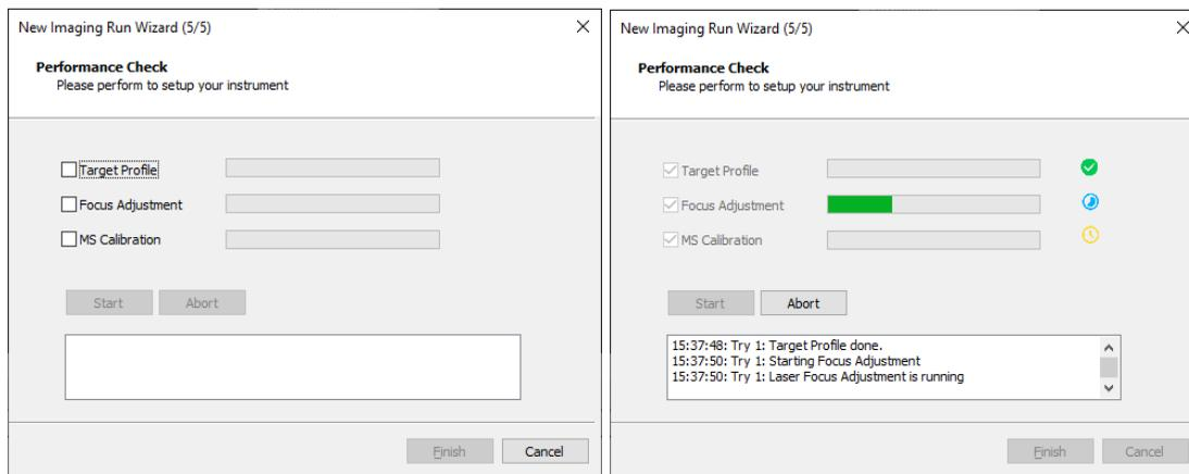
**Figure 5-6** *flexImaging Wizard – Performance Check showing initial settings and completed check*
