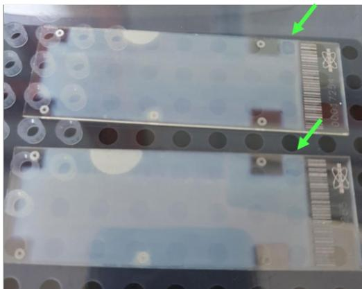
**Figure 3-5** Area for MS calibration, with example of Peptide Calibration Standard II spread in the area.
