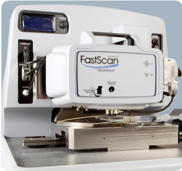
The Dimension FastScan Bio™ Atomic Force Microscope (AFM) enables high-resolution research of biological dynamics, with temporal resolution of up to 3 frames-per-second for live sample observations. What's more, it does this while making the AFM easier to use than ever before.
